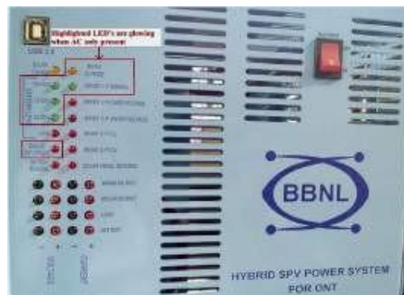
Fig. 3.7.9 Highlighted LED's are glowing when AC only Present
