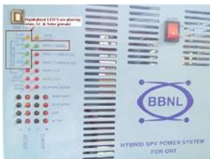
Fig. 3.8.3. Solar &amp; AC Present
