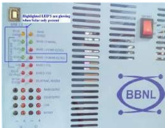
Fig. 3.7.10. Highlighted LED's are glowing when AC & Solar Present
