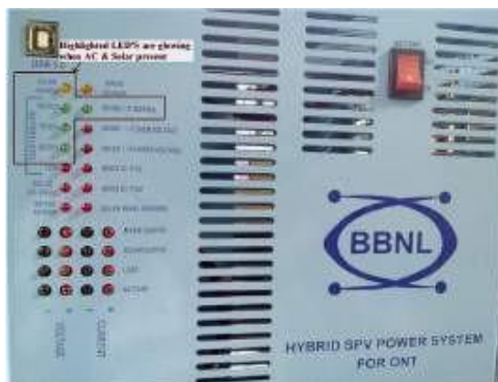
Fig. 3.7.8. Highlighted LED's are glowing when AC & Solar Present
