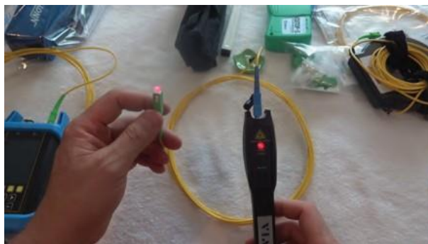
Fig. 6.3.5: Using a Visual Fault Locator (VFL)
