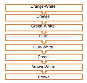
Fig. 2.3.13: Colour code for crimping RJ45 straight cable
