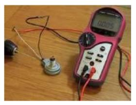
Fig. 2.5.8: Attaching the sensor leads to the multimeter
