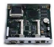
Fig. 1.1.16: Single board computer module
