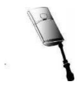
Fig. 2.1.9: Opening the battery cover
