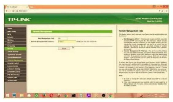
Fig. 2.15.8: Remote management settings for denying any access
