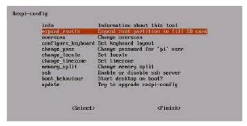
Fig. 2.10.8: A "rasp-config" command
