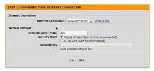
Fig. 2.13.26 (a): Internet connection configuration window
