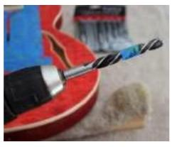
Fig. 2.5.6: Mark the depth of the drill
