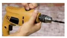
Fig. 2.5.5: Adjust the speed of the drill
