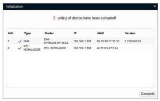
Fig. 2.13.24: Detected devices after initialization
