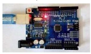
Fig. 1.4.7: Arduino power LED indicator
