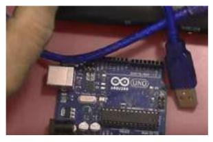
Fig. 2.9.1: Arduino board and cable
