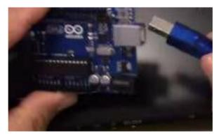
Fig. 2.9.2: Connecting the USB plug to the board
