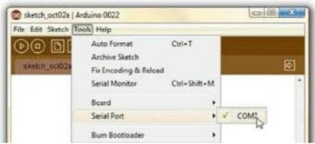
Fig. 2.9.7: Selecting the serial port
