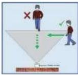
Fig. 2.1.5: Scope of a motion sensor
