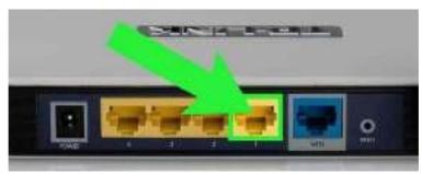
Fig. 2.3.19: Ethernet ports
