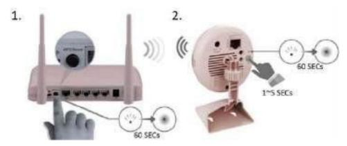
Fig. 5.1.6: Automatic connection of router and camera
