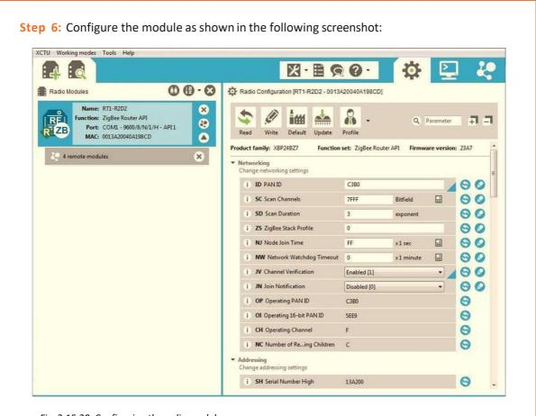
Fig. 2.15.20: Configuring the radio module
