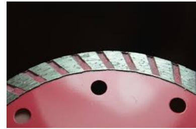
Fig. 4.8: worn out edges of a blade
