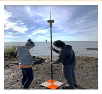
Fig. 3.1.6 typical view of a GCP
