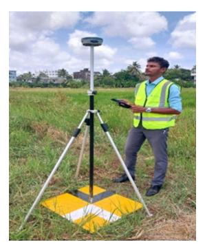
Fig. 3.1.5 Placing GCP
