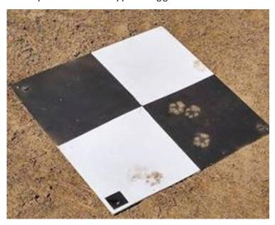
Fig. 3.2.2 Ground Control Points
