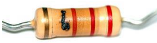
Fig 1.5.8: ESD discharge on a resistor
