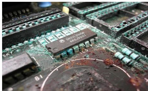
Fig 1.5.6: Metallic filaments on a PCB
