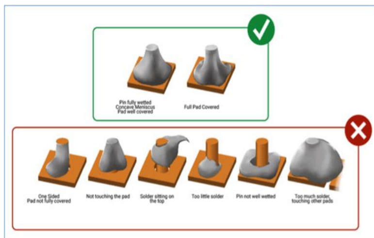
Fig. 5.1.2 Soldering according to J-STD-001 for Soldering
