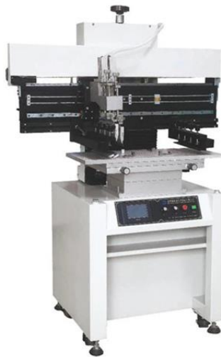
Fig. 2.3.2: A semi-automatic screen-printing machine
