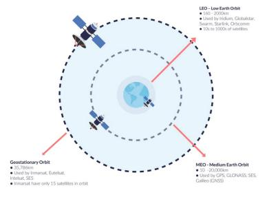
Fig. 3.2.3: How satellite orbit heights impact satellite communication
