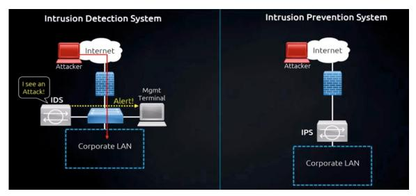
Fig. 4.2.4: Intrusion Detection and Prevention Systems (IDPS)
