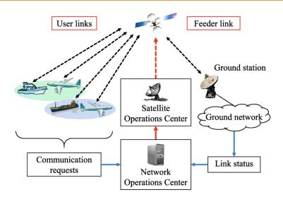
Fig. 1.1.12: SATCOM system and its working
