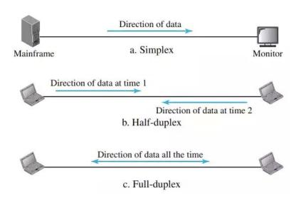
Fig. 2.3.14: Simplex, half-duplex and full-duplex mode
