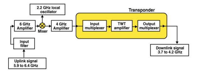
Fig. 1.1.6: Satellite communication block diagram
