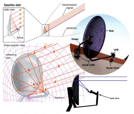
Fig. 2.2.2: How do satellite dishes work?
