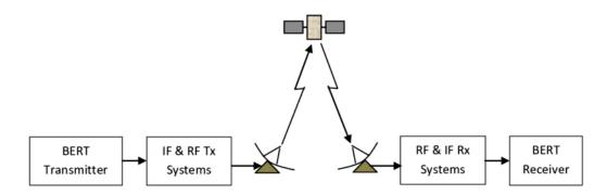
Fig. 4.2.1: BER testing in a satellite communication system
