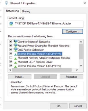
Fig. 2.1.4: IPv4 settings on a laptop
