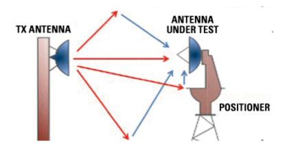
Fig. 2.2.3: Testing of antenna
