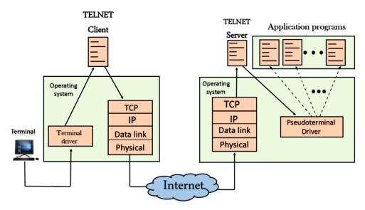
Fig. 2.1.3: Telnet tools in SATCOM operations
