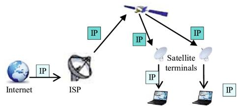
Fig. 7.1.5: Satellite IP Communication System
