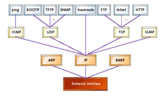
Fig. 3.2.5: How to implement TCP/IP and UDP/IP for embedded systems
