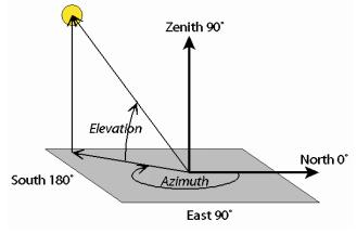
Fig. 2.3.10: Azimuth and elevation" of a satellite
