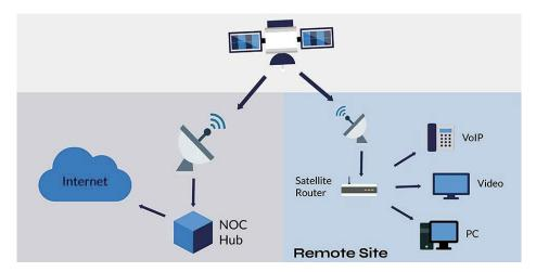
Fig. 5.1.2: How does satellite internet work
