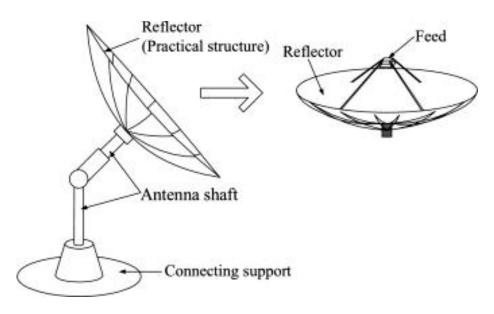
Fig. 2.2.4: Antenna system components
