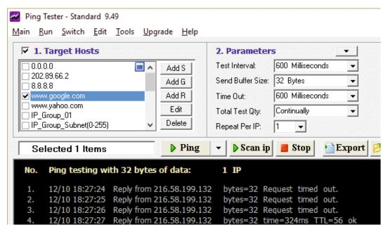
Fig. 6.1.5: Ping tester tool
