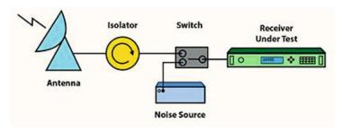
Fig. 2.3.15: Built-in test and calibration
