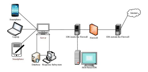
Fig. 3.2.6: A network intrusion detection framework
