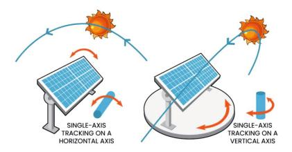
Fig. 3.2.2: Single axis trackers
