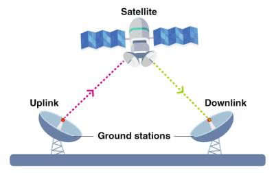
Fig. 1.1.8: One-way satellite communication
