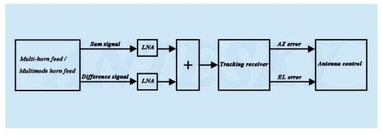
Fig. 3.2.1: Antenna tracking system
