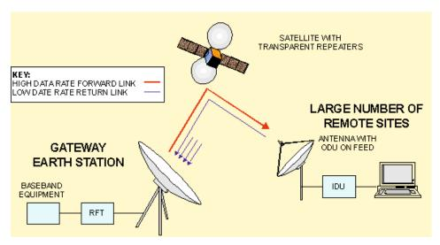
Fig. 2.3.1: IDU in satellite communications
