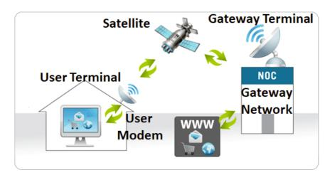
Fig. 5.1.7: Satellite data communication
