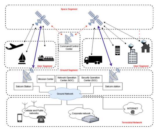
Fig. 6.1.3: SatCom system's communication architecture
