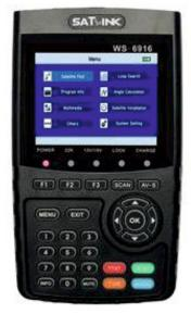
Fig. 2.3.8: Signal strength meter
