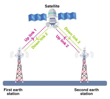
Fig. 1.1.10: Two-way satellite communication
