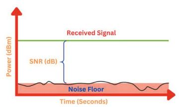
Fig. 2.3.9: Signal-to-Noise Ratio - SNR
