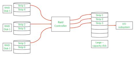
Fig. 5.2.3: RAID (Redundant Arrays of Independent Disks)
