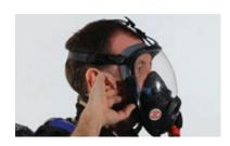
Now insert a finger sidewise of the facemask for easy outward airflow.
