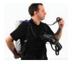
The cylinder valve should be opened slowly to inspect the pressure gauge.
