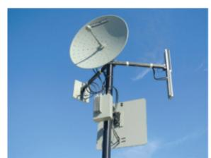
Fig. 1.3.1: Directional Antenna
