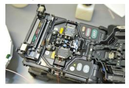
Fig. 5.2.1: Fusion Splicer
