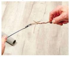
• Strip the insulation from the ends of the cables using a wire stripper.
