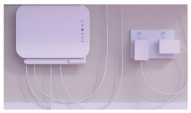
Fig. 5.5.3: Optical Network Terminal (ONT)
