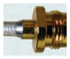
Fig. 7.5.2: Joint after soldering
