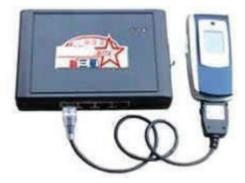
Fig. 8.4.2: Flashing a mobile phone
