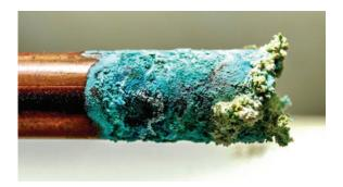
Fig. 9.3.15: Corrosion in Grounding Copper Pipe
