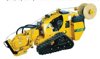
Fig. 3.1.14: Cable Plowing Machine
