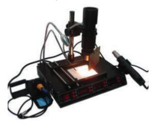
A speedier method, both in setup and heating, an infrared station uses a laser to heat the joint. Therefore, infrared stations are typically more expensive.
