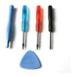
Fig. 8.6.1: Tools required to dismantle a mobile phone
