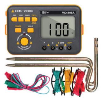
Fig. 9.3.16: Ground Resistance Tester
