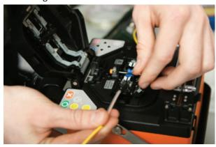
Fig. 3.1.15: Optical Fiber Splicer Machine
