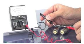
Fig. 3.1.6: Testing of RF cable
