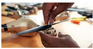
Fig. 2.1.3: Checking propellers of a drone
