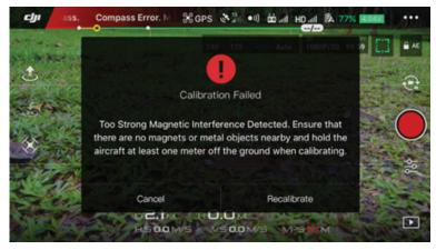
Fig. 4.1.4: Compass calibration error
