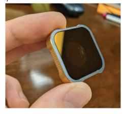
Fig. 4.1.1: Scratches on a ND filter
