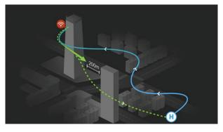
Fig. 1.2.4: Return to home (RTH) feature of a drone
