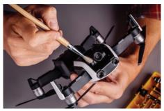
Fig. 4.2.1: Cleaning drone camera with a soft brush
