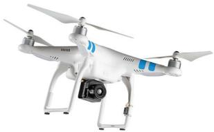
Fig. 5.2.2: Drone fitted with FLIR Vue Pro thermal camera
