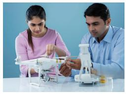
Fig. 4.2.7: Inspecting propellers and motor of drone
