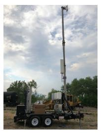
Fig. 2.1.7: Coverage on Wheel or C.O.W
