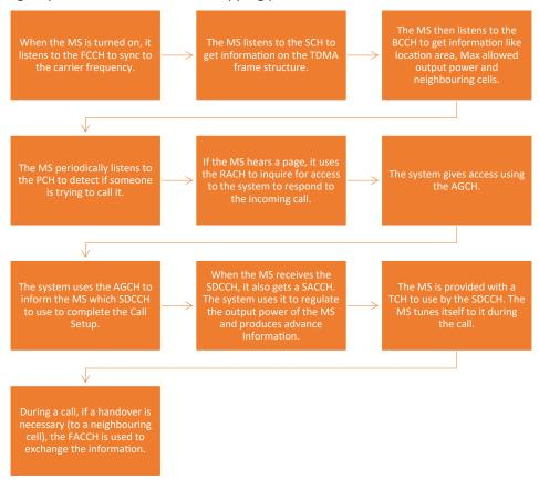
Fig. 1.3.6: GSM Channel Mapping
