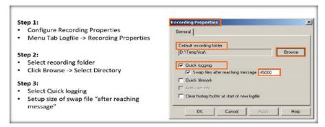
Fig. 4.2.5: Recording in TEMS software
