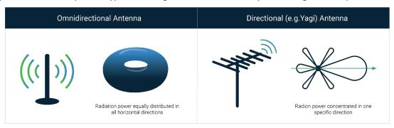
Fig 2.2.1 Types of Antennas used in Cell Towers
