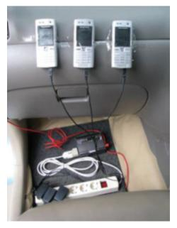
Fig. 3.3.9: A picture taken while conducting drive test
