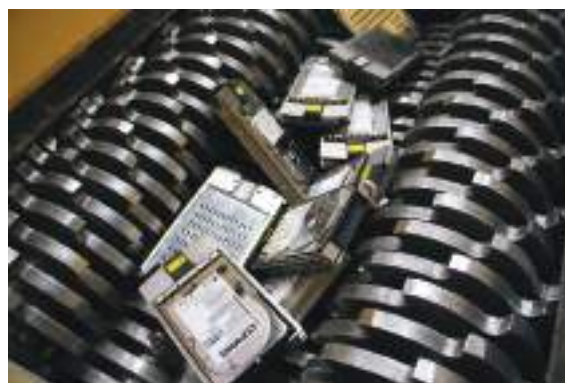
Fig. 2.2.5: Shredding of e-waste using shredder machine
