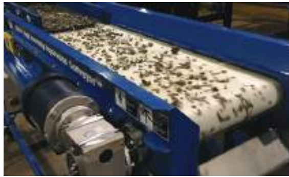
Fig. 2.2.6: Magnetic separator conveyor belt
