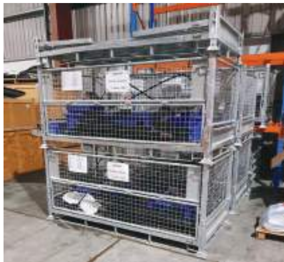
Fig. 2.3.5: Wire Mesh Containers used for storing e-waste
