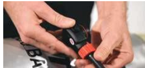
Check the bypass knob (red). Close it if you see it open. After this, press the reset button (area above bypass knob – black)
