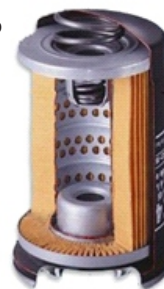
Fig. 2.12.7 Oil Filter and it's construction
