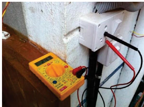
Fig 5.2.5: Connect black test probe to earth outlet
