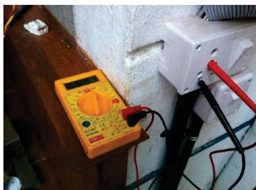
Fig 5.2.6: Red probe and black in earth and neutral respectively
