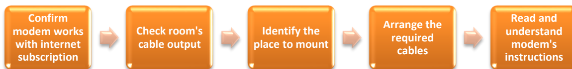
Fig 2.4.1: Items to be checked before installing modem
