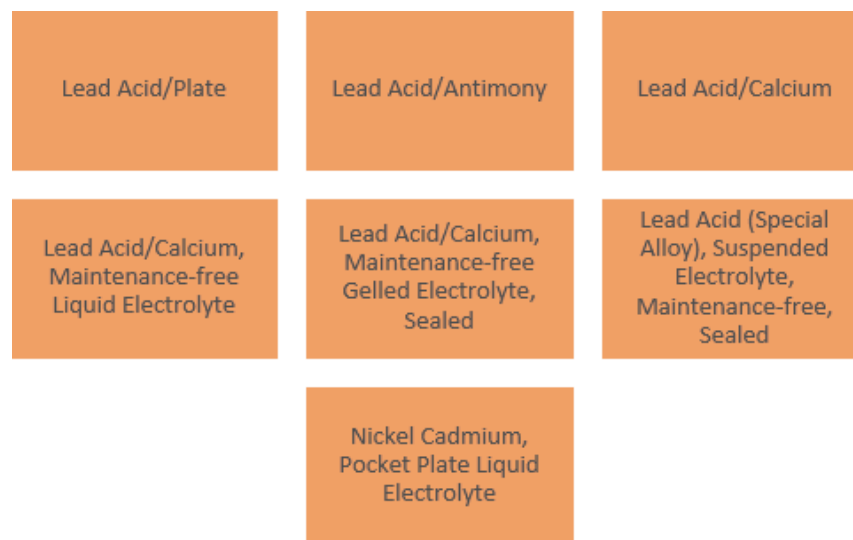
Fig. 5.6.1: Batteries, used for UPS
