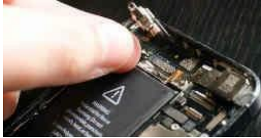
Fig. 2.6.8: A faulty vibrator
