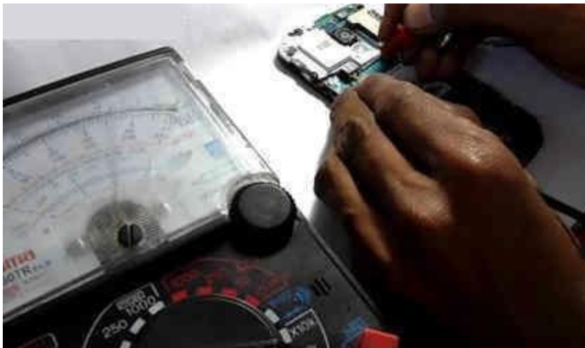
Fig. 2.5.6.3: Checking shorting with multimeter
