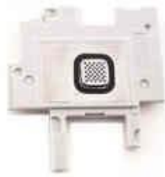
Fig. 2.6.7: A faulty ringer
