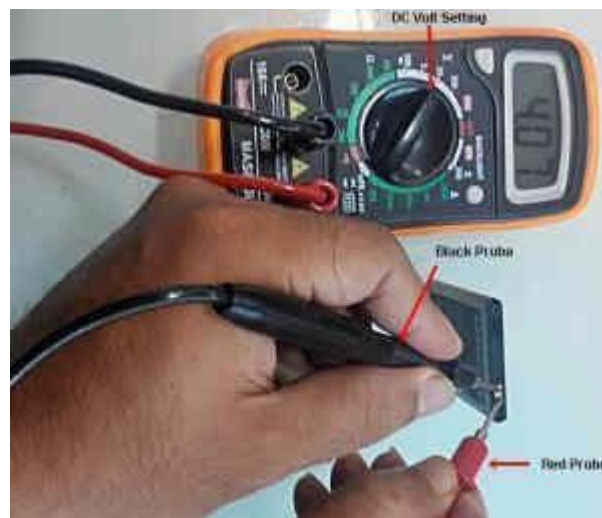
Fig. 2.5.6.1: Checking the battery with a multimeter
