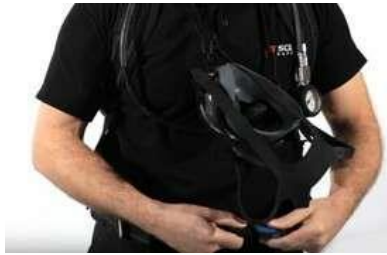
After wearing the breathing apparatus tighten shoulder straps and fasten the waist belt.
