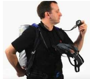
The cylinder valve should be opened slowly to inspect the pressure gauge.
