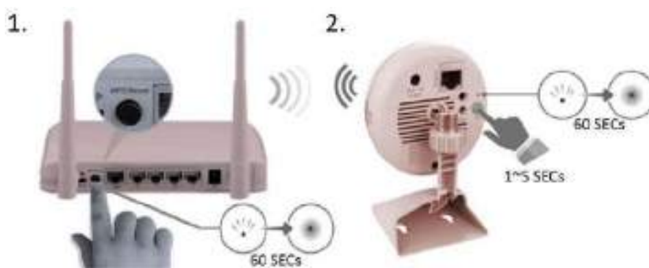
Fig. 5.1.6: Automatic connection of router and camera
