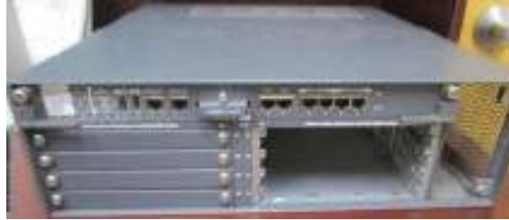
Fig. 2.2.6: A metal enclosure for the gateway
