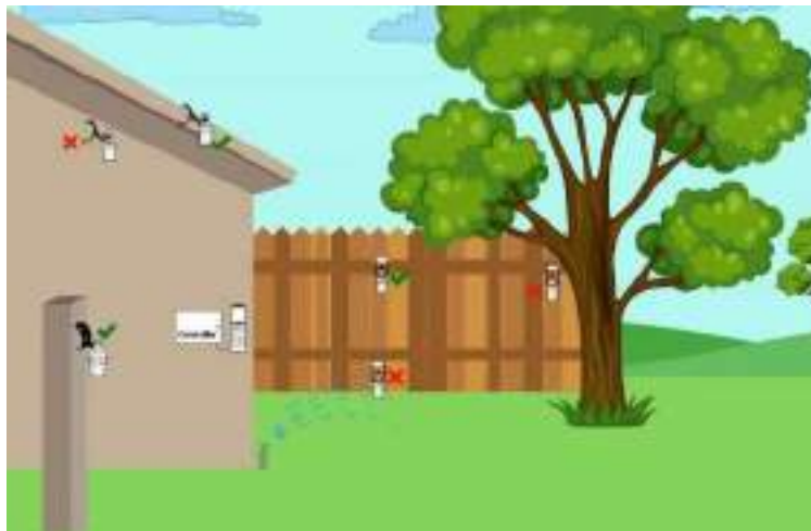
Fig. 2.1.4: Suitable location for outdoor sensors
