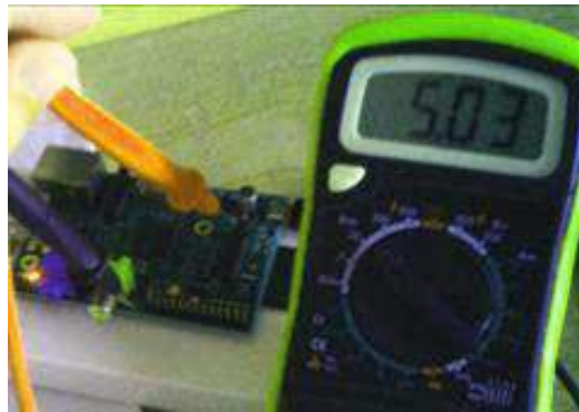
Fig. 6.5.7: Power supply testing in power down mode
