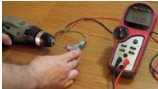
Fig. 2.5.9: Increased voltage output of the sensor with increased RPM of the drill
