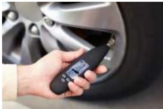
Fig. 1.2.3: Measuring the air pressure of tyre using pressure sensor
