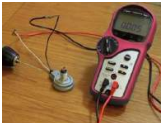
Fig. 2.5.8: Attaching the sensor leads to the multimeter
