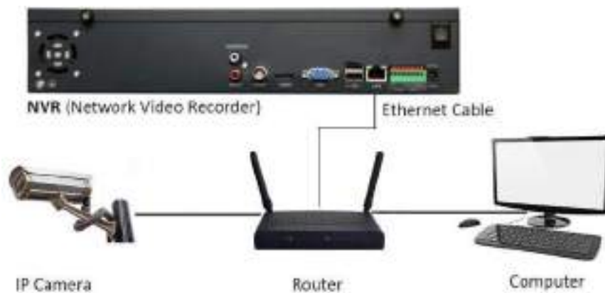
Fig. 2.13.18: NVR device connection with router and camera
