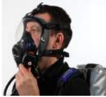
Normally Breathe to vent system Listen for a whistle alarm while observing the pressure gauge at 55 bar (+/-5 bar)
