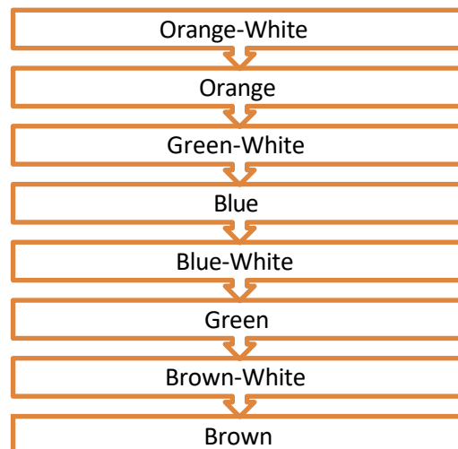
Fig. 2.3.13: Colour code for crimping RJ45 straight cable
