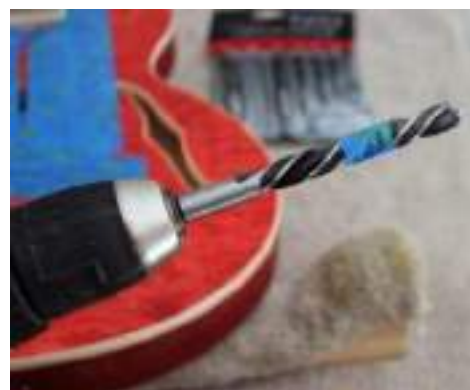
Fig. 2.5.6: Mark the depth of the drill
