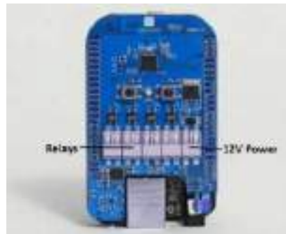
Fig. 2.2.9: A relay module to be connected to the gateway
