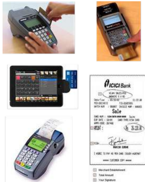
Fig. 2.2.2: EDC machine or Card swipe Machine & Sample Receipt Or Sample Merchant copy
