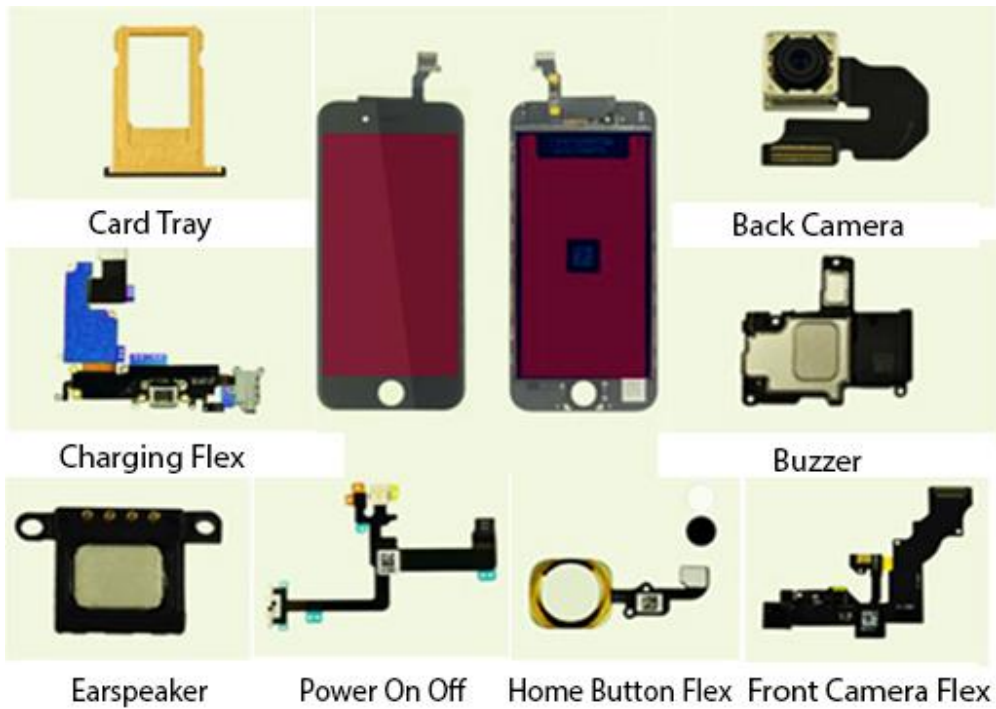
Fig 1.5.1: Basic parts of a mobile phone
